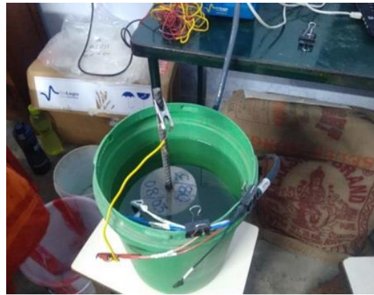
Figure 4.1 Corrosion test set up
