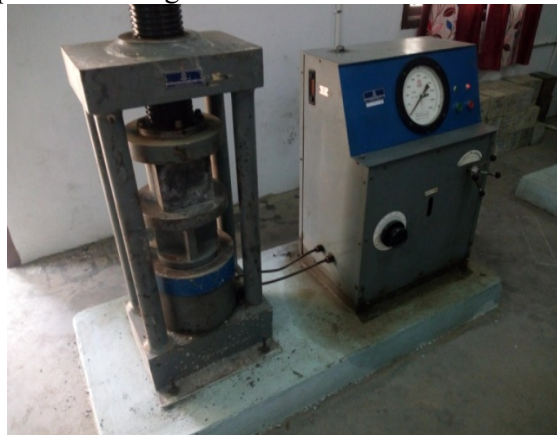
Fig 5. Testing of GPC Cube Test in CTM
