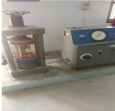
Fig 11, Compression Test of Cylinder Specimens
