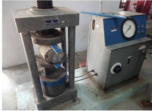
Fig 8. Testing of cylinder specimen using split tensile in compression
