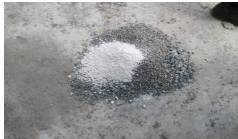
Figure 4. Dry Mix of GPC with Granite Powder
